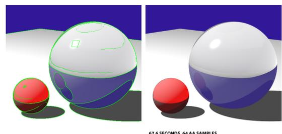
Figure 2: Using the corner-point method for AA sampling we were able to perfectly target aliased regions using an  $\epsilon$  of 0.01 leading to a 500x500 render with a max depth of 64 AA samples being rendered in 67.6 seconds
